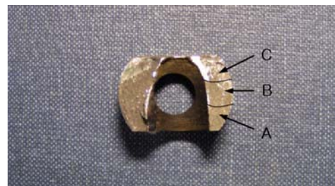
(b) Fractured surface of rocker arm shaft
