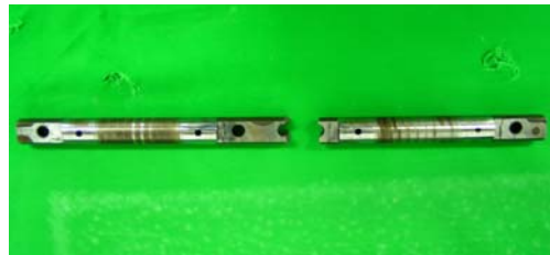
(a) Failure of rocker arm shaft in the 4-Cylinder SOHC engine
